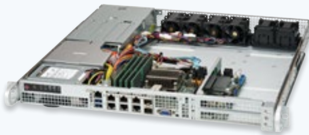
X10SDV-7TP8F 9" X 7.25" Flex ATX Front I/O
