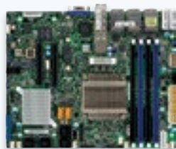
X10SDV-7TP8F 9" X 7.25" Flex ATX Front I/O
